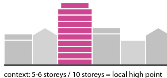
Figure 1.1: A 10 storey building is perceived as tall in a 2-storey context while in an urban 5-6 storeys context is only considered a local highpoint
